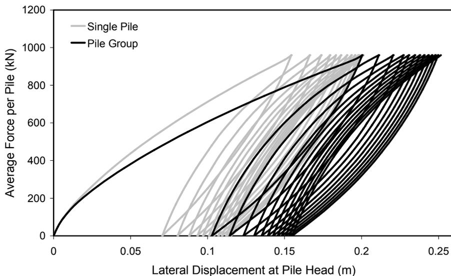
Figure 6. Force – Displacement curve of the single pile and the pile group for the loading of test P344
