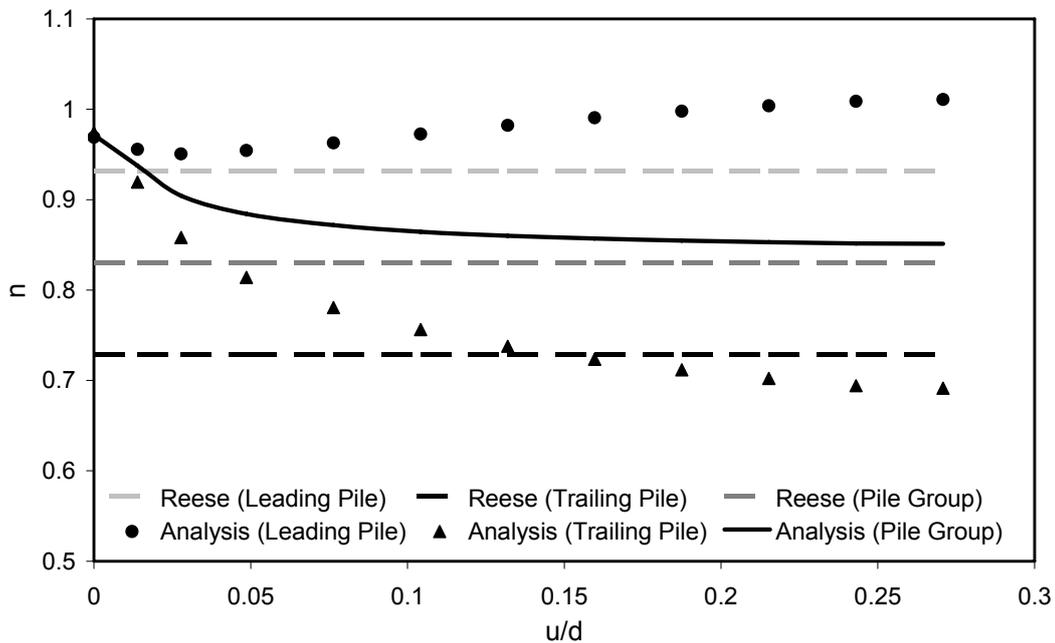
Figure 9. Comparison of efficiency factors of the numerical analysis with the efficiency factors proposed by Reese and Van Impe.
