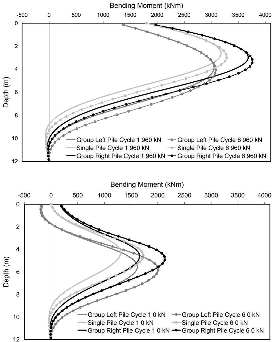
Figure 7. Comparison of computed bending moment distributions of the pile group and the single pile for test P344 at two different stages of loading : a) at the 1st cycle, and b) at the 6th cycle. The maximum applied load is 960 kN and the minimum load is 0 kN.
