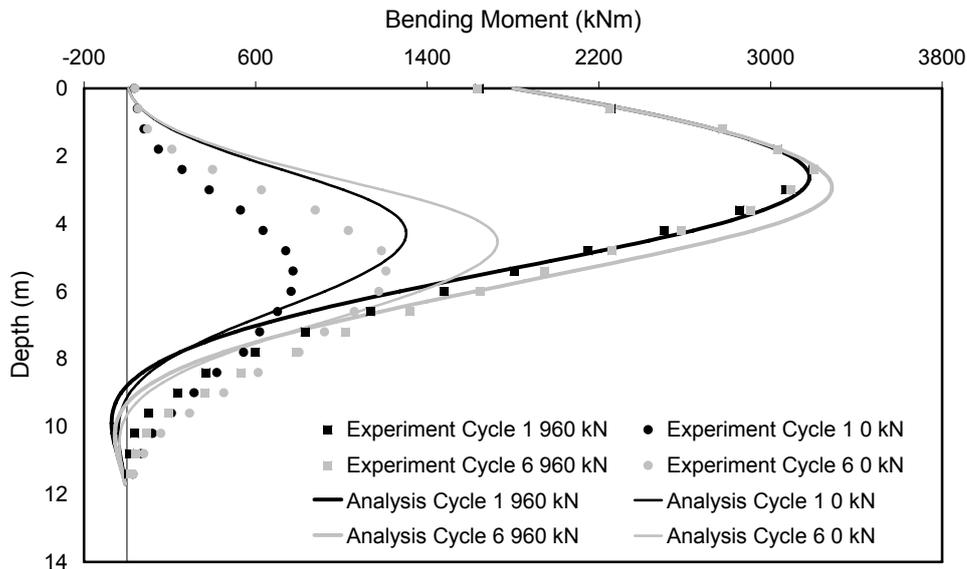
Figure 4. Comparison of computed and recorded bending moment distributions for test P344 at two different stages of loading : a) at the 1st cycle, and b) at the 6th cycle. The maximum applied load is 960 kN and the minimum load is 0 kN.
