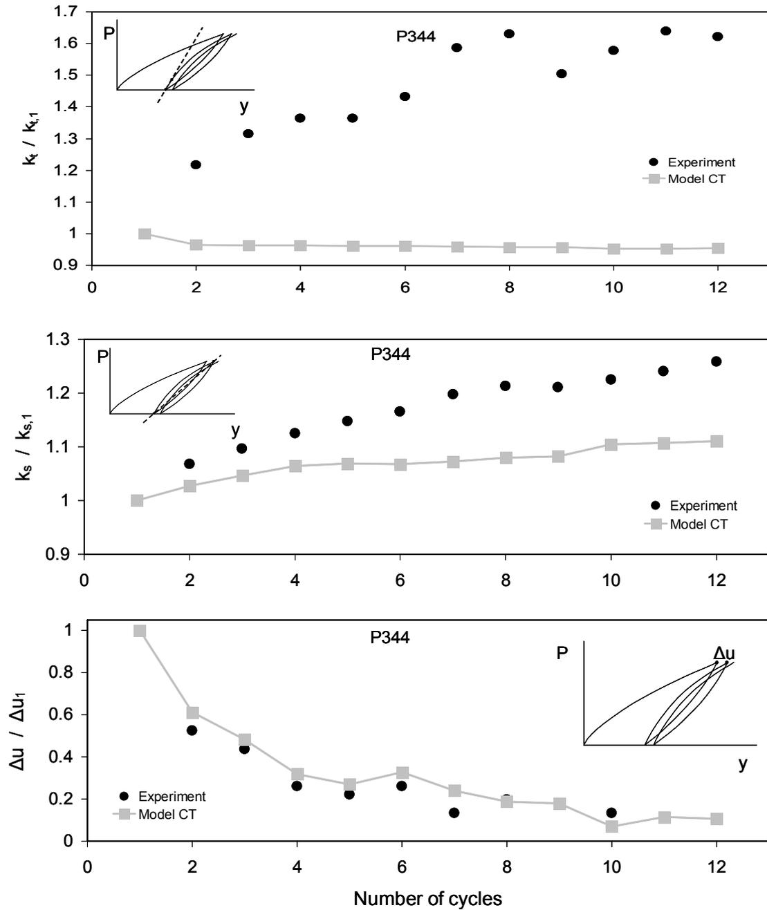
Figure 5. a) Normalized tangent stiffness with respect to the first cycle of loading, b) Normalized secant horizontal pile stiffness with respect to the first cycle of loading, c) Relative pile-head displacement between two consecutive re-loading–unloading reversal points normalized with the one between the loading-unloading and the first re-loading – unloading reversal points
