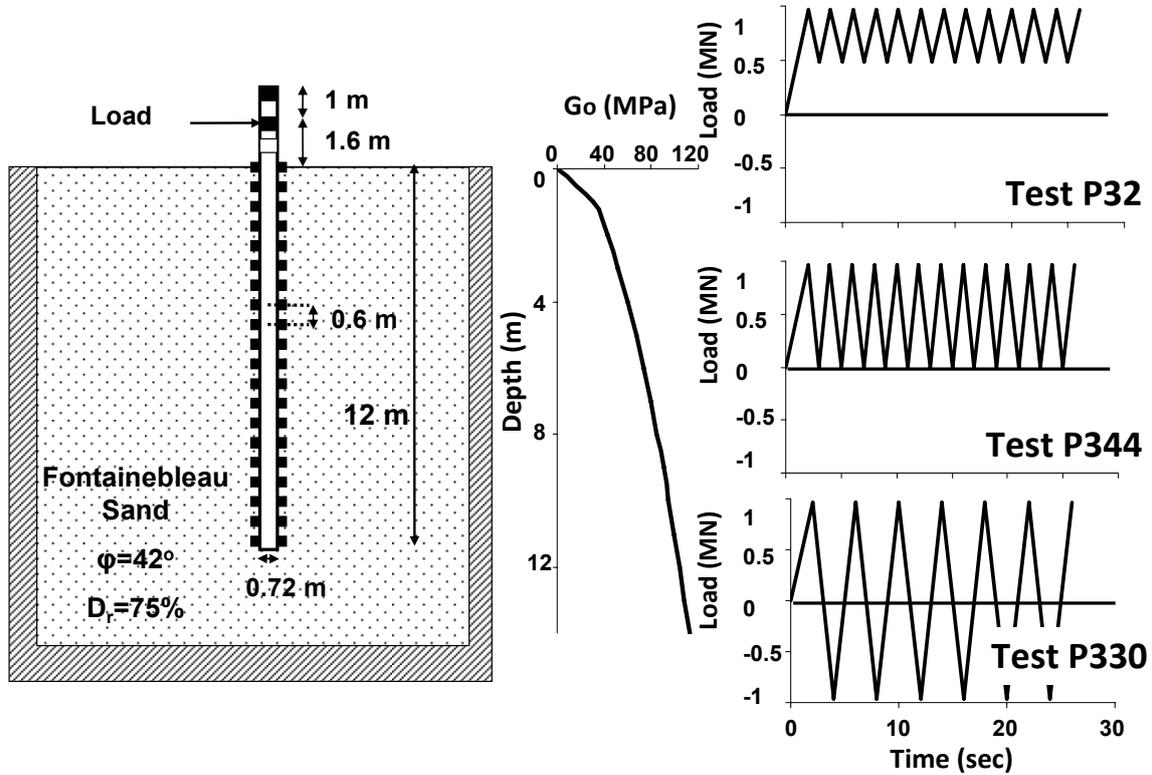
Figure 1. Experimental setup of the centrifuge tests conducted in LCPC (Rosquoët et al, 2004) and load time histories of the three tests (P32, P344 and P330). All dimensions refer to the modeled prototype
