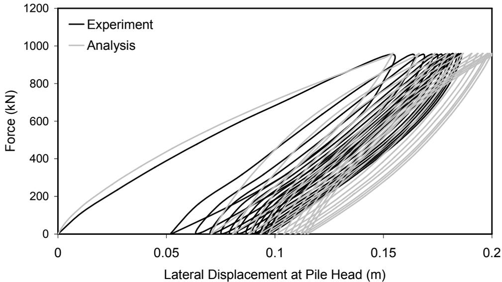
Figure 3. Experimental and Computed Force – Displacement curve at pile head for single pile
